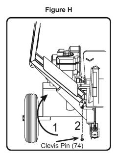
Raise the Log Lift and insert the Clevis Pin (74) in the upper hole and secure with R-pin (41) - See Figure H.
